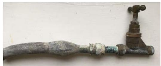
A lead pipe showing a swollen 'lead wipe' joint
